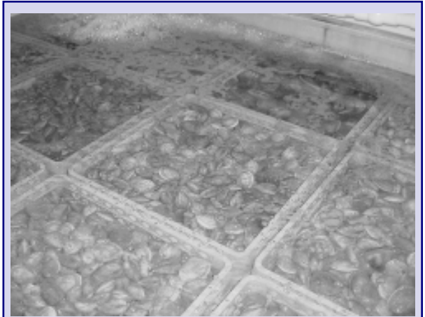
Clams undergoing purification at a depuration facility, the Clean Water Clam Plant in Sea Bright NJ, the region's original plant.
